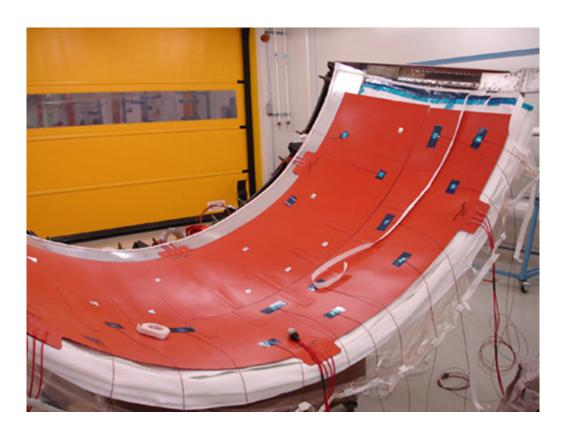
GMI has developed several solutions during the last twenty years to repair reversers on various engines, the main task being the wiremesh full reskining of Transcowls and Corecowls. With the time and according to the volume of business of various customers different solutions can be proposed :
