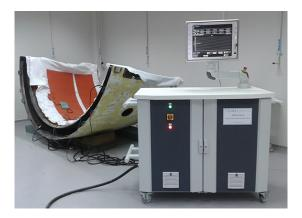
The complete equipment that will control and power the heating blankets is organized in a rolling bench . The equipment is composed of :
