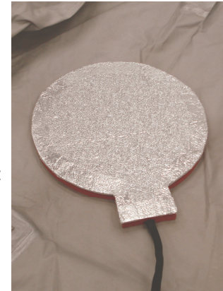
Figure 2: Heating circuit with special protective upper support
