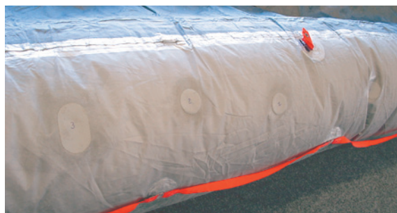
Figure 3: View of repair patches
