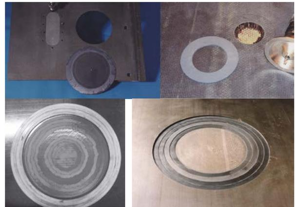
**Figure 3:** Illustration of routing, scarfing and stepping operations
