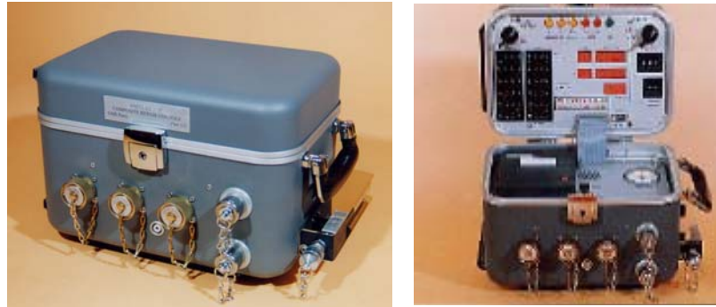
Figure 1: On left, the Anita OT closed showing external connectors of high quality. When opened (right) the Anita appears straightforward to be used; no complicated keyboard; a software has been designed so that the ANITA answers automatically to switch selections .
