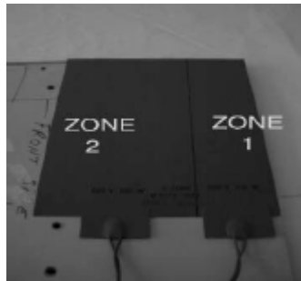
Figure 2: Here a blanket with two circuits to control differently two adjacent areas: one being a uniform laminate, the other with stringer constituting a heat sink.
