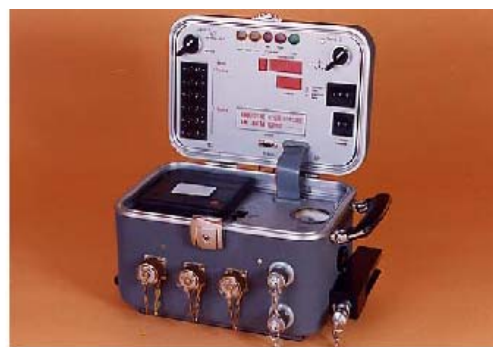
Figure 1: On left, the Anita NG closed showing external connectors of high quality When opened (right) the Anita appears straightforward to be used ; no complicated keyboard ; a software has been designed so that the ANITA answers automatically to switch selections.
