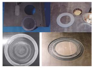
Figure 3: Illustration of routing, scarfing and stepping operations
